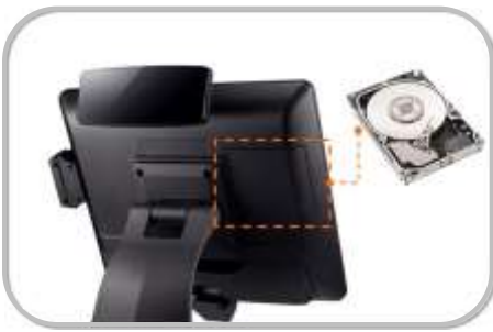
Easy access 2.5" HDD for installation and maintenance
